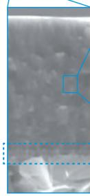
**Our proprietary super multi-layered coating structure:** Advanced nanotechnology enables nanometre-level thickness (1 nanometre is one billionth of a metre). Hardness, thermal resistance and toughness are significantly improved by alternately layering one thousand layers of super thin film
