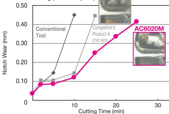
Work Material: SUS316L Insert: CNMG120408N-GU
