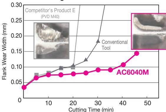
Work Material: SUS316 Insert: CNMG120408N-GU
