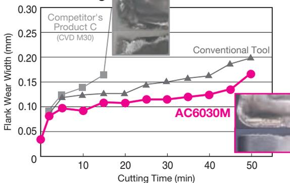
Work Material: SUS316 Insert: CNMG120408N-EX
