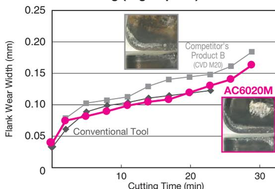
Work Material: SUS316L Insert: CNMG120408N-GU
