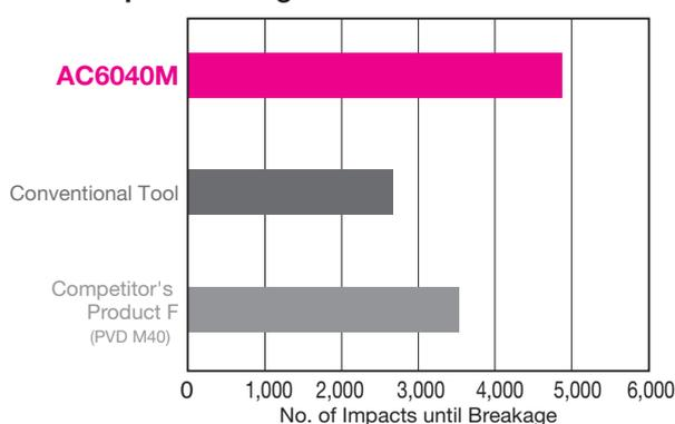
Work Material: SUS316 Insert: CNMG120408N-GU
